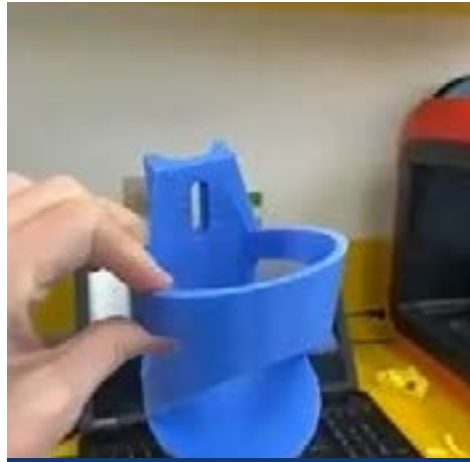
An adapted cup holder for a wheelchair or walker designed using Dana Point MTU's 3D printer.
